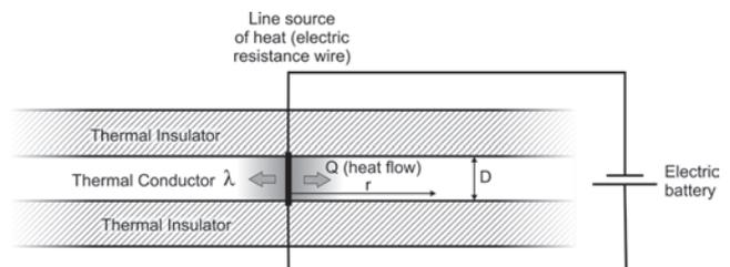
Fig. 6 - A conceptualisation of Horatio Scott Carslaw's line heat source in an infinite conducting plate. Slightly modified after Banks (2012) (© John Wiley & Sons, Chichester 2012).
