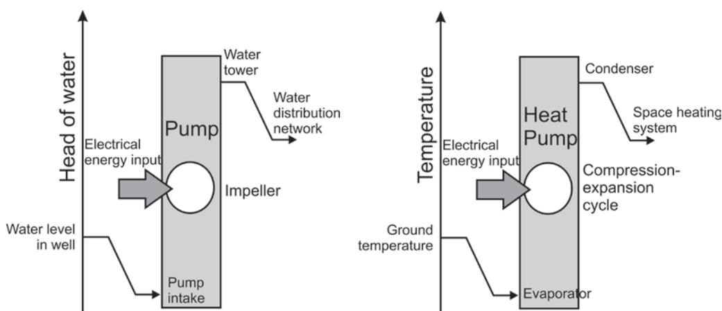
Fig. 2 - Conceptualisation of the analogies between an electrical centrifugal water pump and an electrical compression-expansion cycle heat pump.
