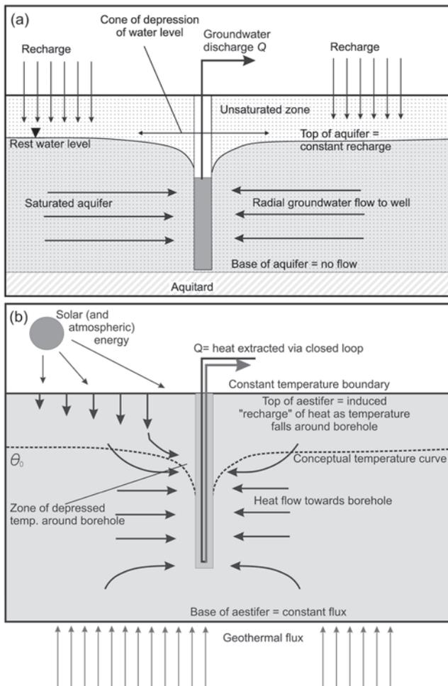
Fig. 7 - Comparison of conceptual models, with upper and lower boundary conditions, for (a) a well in an unconfined aquifer and (b) a closed loop borehole heat exchanger in a typical aestifer.  $\theta_0$  is the undisturbed "rest" temperature in the aestifer. Slightly modified after Banks (2012) (© John Wiley & Sons, Chichester 2012).
