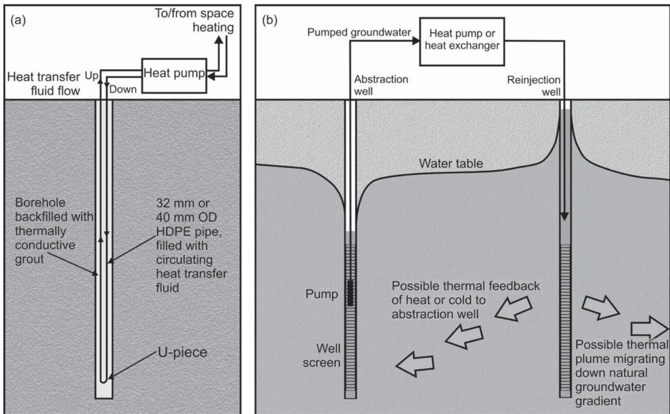
Fig. 4 - Schematic diagrams of (a) a closed-loop borehole heat exchanger ground source heat pump system and (b) a well-doublet open-loop ground source heating or cooling system. HDPE = high density polyethylene, OD = outside diameter.
