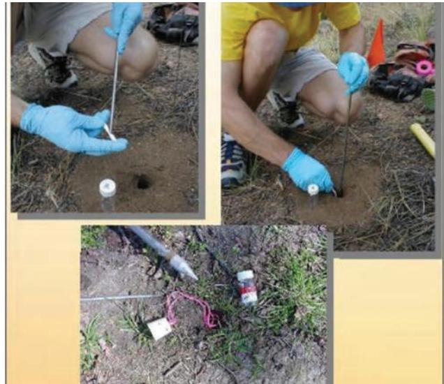
Fig. 5 - Passive soil gas samplers. Field examples of installation procedure.
