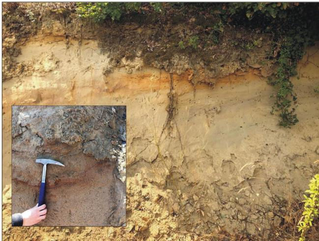
Fig. 2 - Detail of the outcropping of SC soil.
