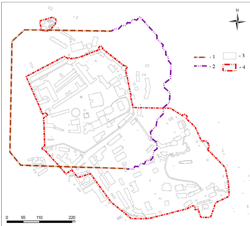
Fig. S7 - The filtration domain and boundary conditions of the groundwater flow model.
