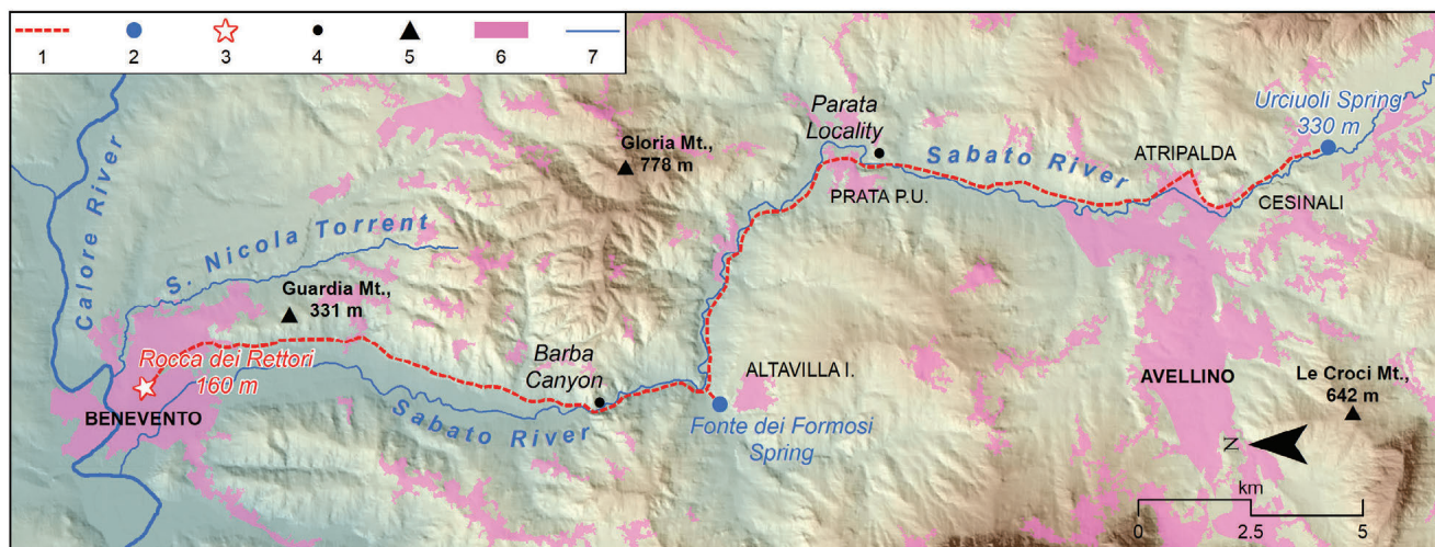
Fig. 2 - Map showing the path of the Roman Aqueduct (I Century A.C.) conveying waters of the Urciuoli karst spring to Benevento city. Legend: 1) Hypothesized Aqueduct path; 2) Main springs; 3) Castellum Aquae (Rocca dei Rettori); 4) Main toponyms; 5) Mountain peak; 6) Towns; 7) River network.
