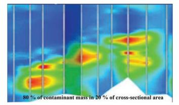
Fig. 2 - Transect perpendicular to groundwater flow direction. The figure shows that most of the contamination is located in limited soil volumes.
