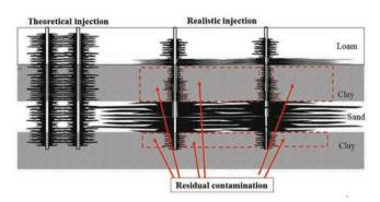
Fig. 4 – Differences between theoretical and actual injection radius due to soil beterogeneities. Different injection radii are actually obtained due to soil beterogeneities (the lower the permeability, the smaller the radius of influence), thus leading to incomplete remediation of target areas.
