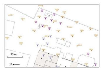
Fig. 11 - Location of MIP points and passive soil gas samplers in the Eastern site sector. Purple points show the MIP locations; a total of 8 MIP points was located in the Eastern site sector. Orange crosses show the passive soil gas samplers location. Points named "Cr..." are soil borings not described in the present article.
