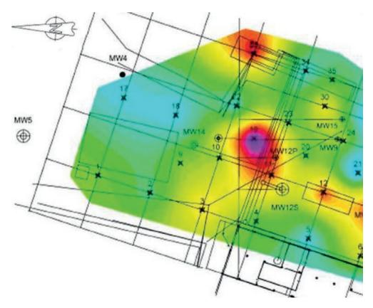
Fig. 14 - TPH – Soil gas passive samplers results in the North-Eastern site sector. The main TPH impact detected by the passive soil gas sampler n. 19 (whose location is shown in Figure 11 as "GS19", near MIP point V13) is shown in purple.
