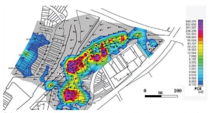
Fig. 6 - Passive soil gas samplers – Typical results of the investigation. The most impacted areas are shown in purple. Passive soil gas sampling data are reported in units of mass (as shown in the column on the right sector of figure), although concentration data can be in some cases calculated.
