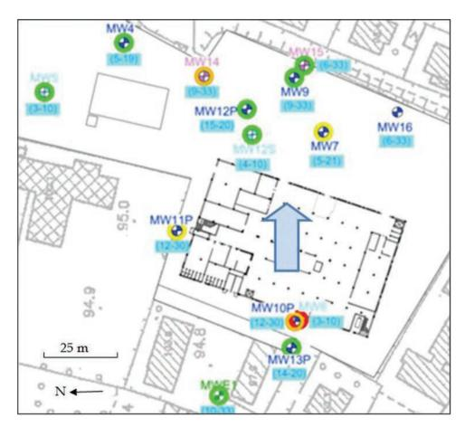
Fig. 8 - Site Groundwater Impacts. Monitoring wells (MW) names are shown (screened intervals in m bgl are reported in round brackets). Chlorinated impacts are shown in green (<10 µg/l), yellow (10-100 µg/l), orange (100-1000 µg/l), purple (1,000-10,000 µg/l) and red (> 10,000 µg/l) circles. Main groundwater flow is West-East. MW14 and MW15 are bydraulic barrier wells. The main production building is located just East of monitoring wells MW6 and MW10P.
