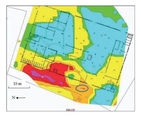
Fig. 13 - Western Site Area - 2D Interpretation of CHC Main Subsoil Source Areas at 2 m bgl. Main CHC subsoil impacts identified by the DELCD sensor at 2 m bgl are shown in purple and red. The location of the most impacted monitoring wells MW6 and MW10P is shown in the blue circle right of the most impacted subsoil area.
