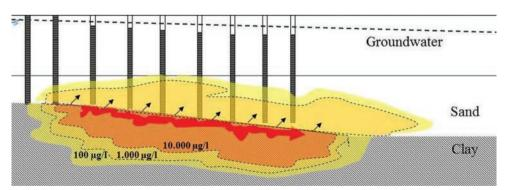
Fig. 3 - Rebound effect from low-permeability layers after remediation of bigb-permeability layers. If remediation activities are focused on bigb-permeability layers only, dissolution of residual contamination located in low-permeability layers may generate rebound effects.
